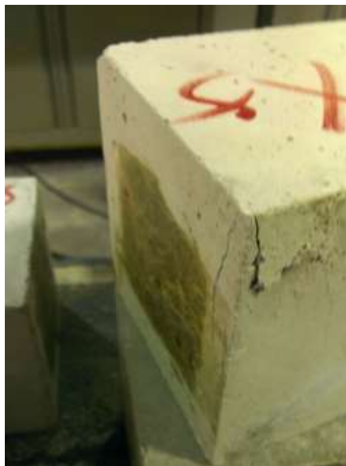
Picture 3.4.2.2- A record of failure form of a specimen after compression test
