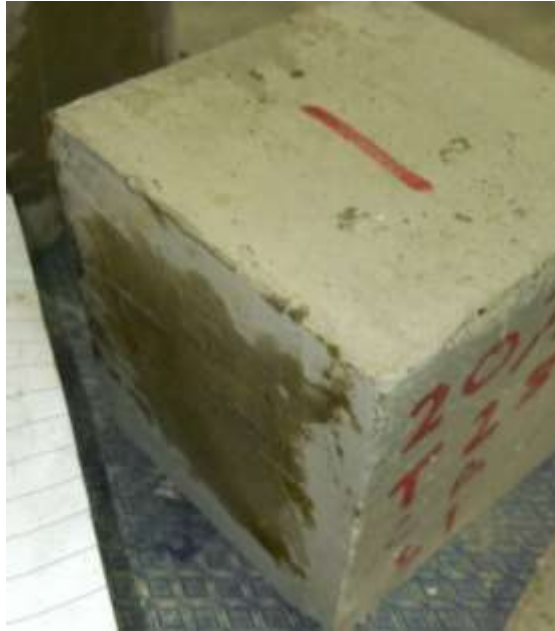
Figure 3.6.3.2-The surface that was applied with couplant
