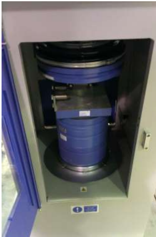
Picture 3.4.2.1-Inside of a compressive strength test machine
