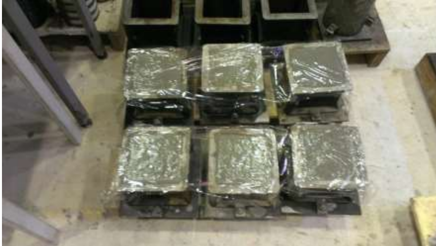
Picture 2.3.3.1-The molds were covered by plastic sheets
